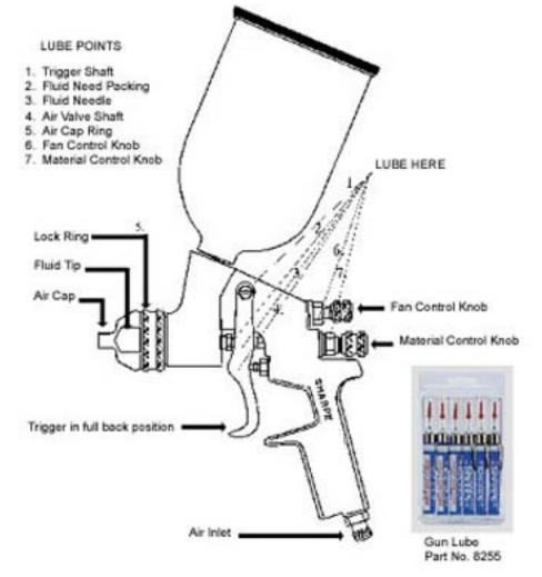
1. The spray gun should be lubricated after every cleaning using SHARPE gun lube. Place a drop on all moving parts, as shown in illustration.
