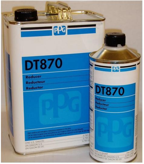
A reducers main purpose is to make the paint thin enough to spray through a gun as well as providing leveling of the paint and adhesion. They are made up of a combination or blend of different solvents. The blends are different depending on the conditions and temperature. By using the wrong reducers, you can get everything from runs and sags to orange peel, if it does not flash off at the correct speed. Below is a list of recommended temperature ranges for Urethane reducers.
